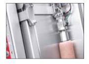
The patented vacuum gripper (optional) securely holds soft products such as boiled sausage, thereby ensuring reliability of the production process.
