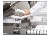
Easy handling to the last detail: The cutting frame can be removed manually in just a few steps.
