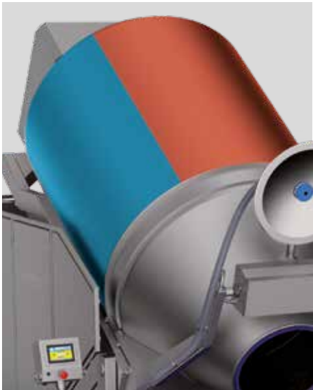
Refrigerated-heated jacketing with automatic thermal control
