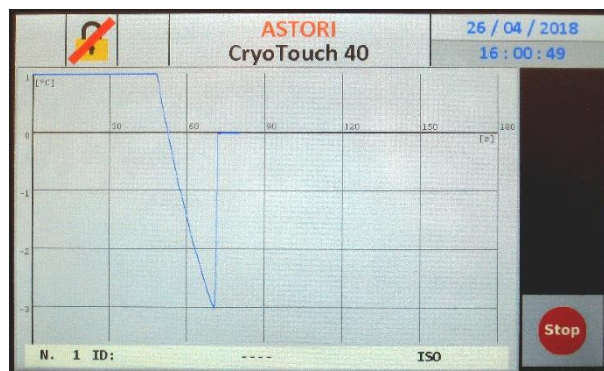
Real-time graph of the cryoscopic point measurement
