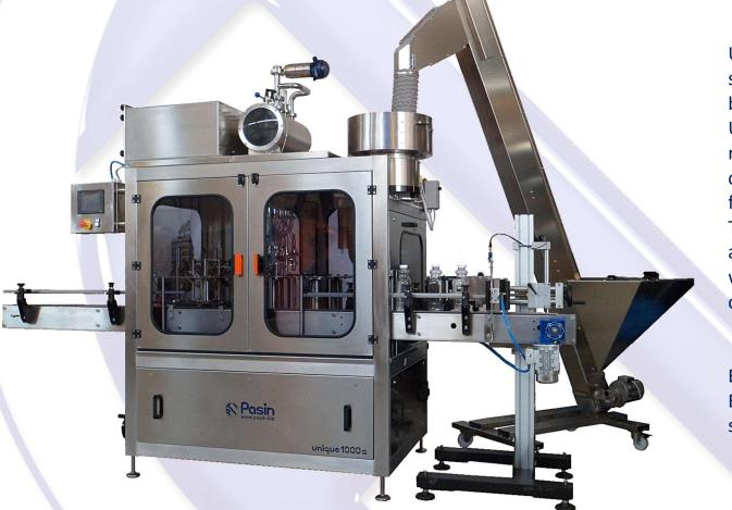
UNIQUE stands for a group of mediumspeed packaging machines, suitable for bottling liquid or semiliquid foodstuff. Unique is composed of a series of rotative carousel mechanically connected together, proper for rinsing, filling and capping bottles.
