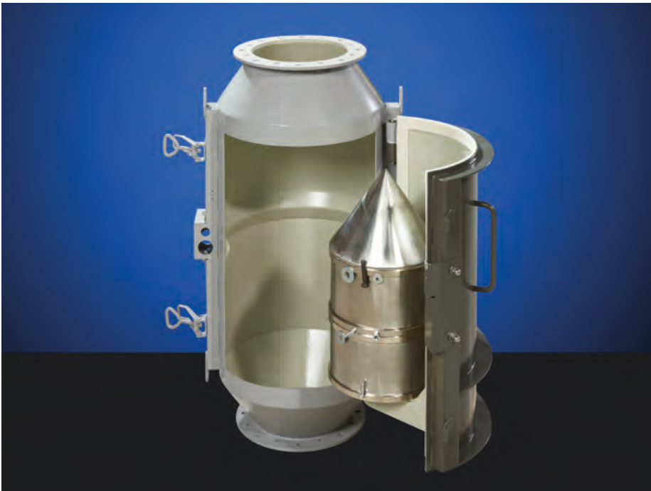
Bullet magnet for ceramic material
