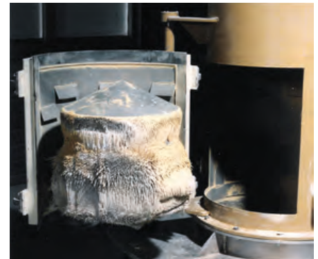
Bullet magnet for ceramic material
