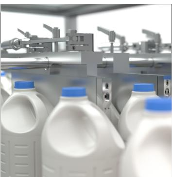
The products, according to their characteristics and operating speed, are stored and composed in the requested configuration in order to be picked up in the desired quantity and subsequently deposited inside the crates.
