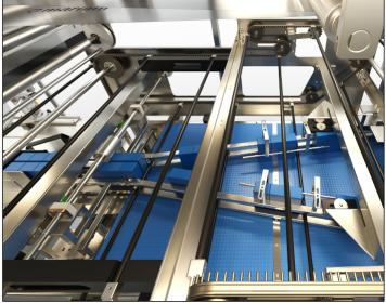
Packs, during the feeding cycle, are wrapped in film before they enter the shrink-tunnel resulting in a tightly wrappped final bundle. This operation is done by a cut and seal unit that ensure the perfect clusure of the bundles.
